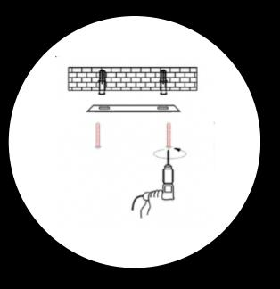
THE HANGING PLATE IS INSTALLED FIXED TO THE WALL
